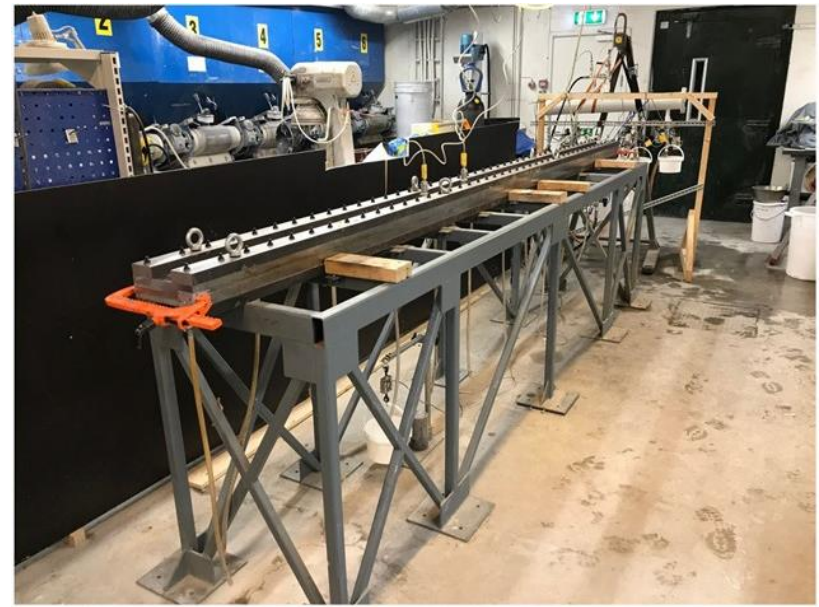
Variable Aperture Long Slot (VALS) and dynamic injection unit at laboratory
