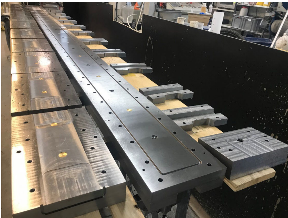
New design of Variable Aperture Long Slot (VALS) with possibility to change order of apertures.
