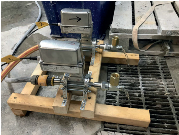
Figure 17. The flow meter connected to tap water hoses to test reliability of the signal conversion and the DAQ system.
