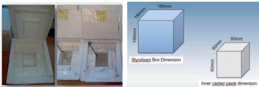
Figure 12. Semi adiabatic temperature measurements setup
