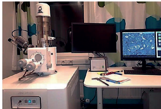
Figure 13. Scanning electron microscope (SEM) integrated with an energy dispersive spectrometer (EDS) used for the characterization of microstructure and phase composition.
