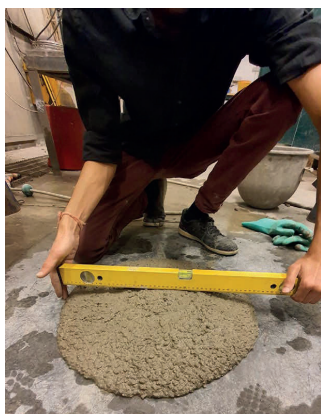
Figure 15. Example slump and slump flow tests of a) ANL OPC:BELI_80:20 b) OPC:BELI_60:40
