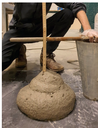
Figure 15. Example slump and slump flow tests of a) ANL OPC:BELI_80:20 b) OPC:BELI_60:40
