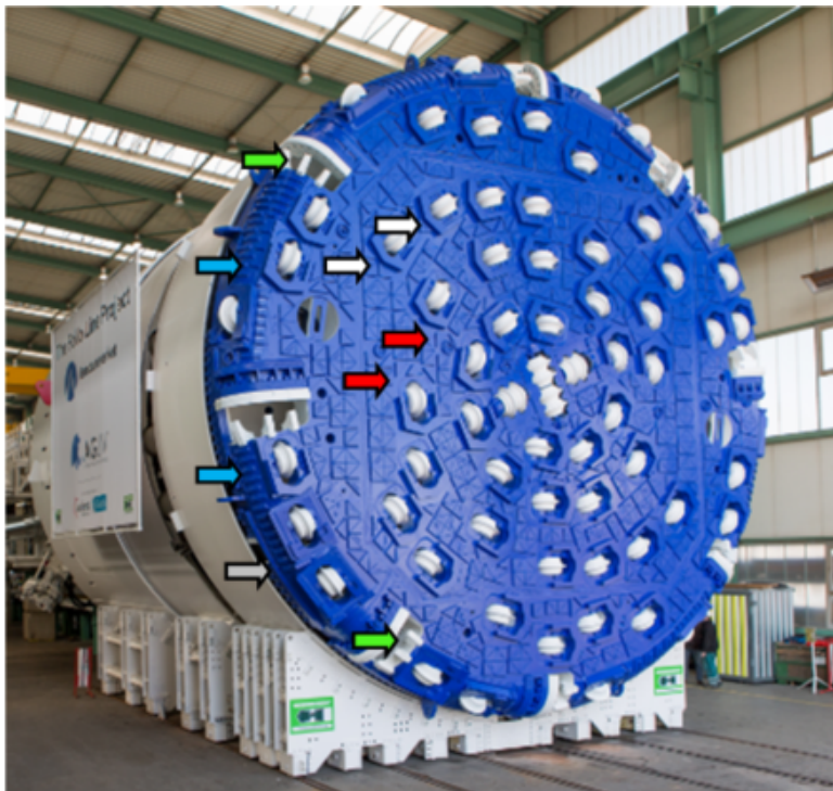
Figure 2. Wear protection features and details on the original Follo Line cutterhead Wear protection on the cutterhead: ⇨ Wedges to protect the cutters; ⇨ Wear plates for the face; ⇨ Wear protection at cutterhead periphery; ⇨ Grillbars to protect the cutterhead periphery; ⇨ Calibration-bars to protect the scrapers from big blocks and control maximum block size to enter the cutterhead
