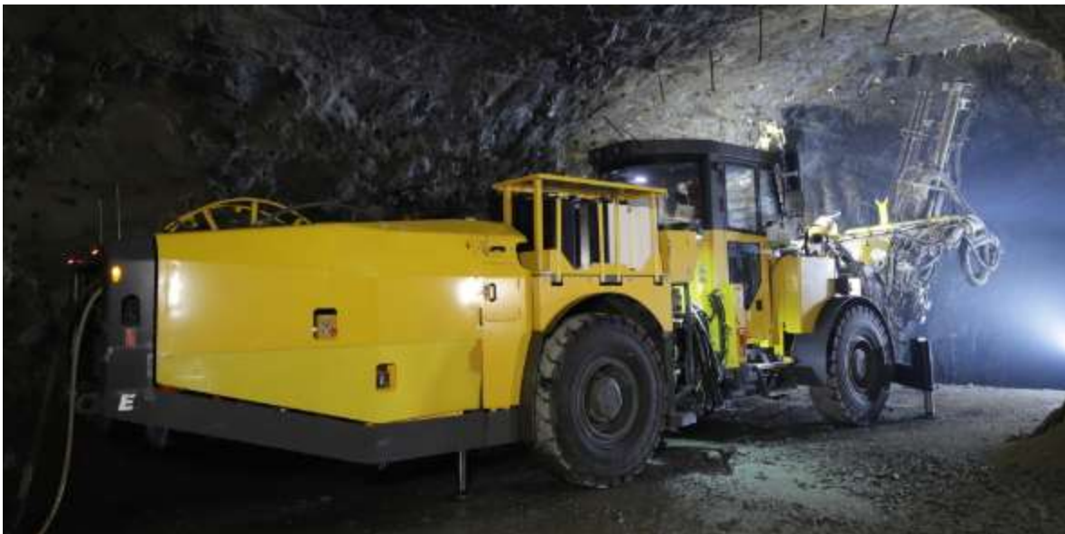
Figure 14. The containers for components A and component B on-board the rig.
