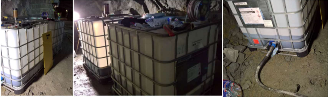
Figure 13. IBC containers (1 m 3 each) for components A and B that are used to refill the on-board tanks. (LKAB)
