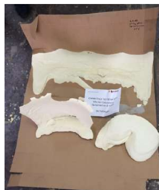
Figure 6. Shows an early test of pumpable resin to explore it's properties (Minova)
