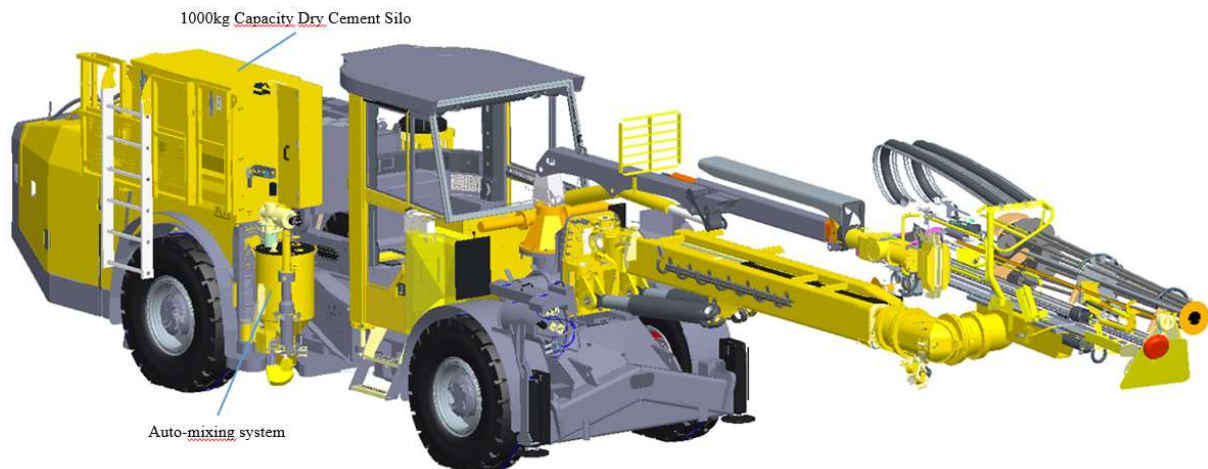
Figure 1. Boltec EC with Auto-mix cement grout system
