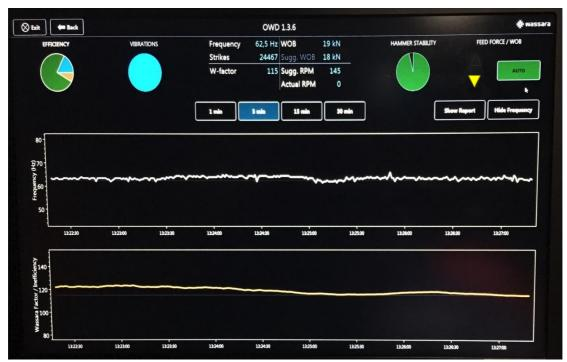
Figure 4. LKAB Wassara OWD® in action keeping hammer frequency constant and in range while gradually reducing drilling inefficiency parameter Wf.
