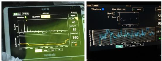
*Figure 2. LKAB Wassara OWD*® *stand-alone unit in open-loop mode and its closed-loop counterpart in auto mode continuously regulating rig parameters.*
