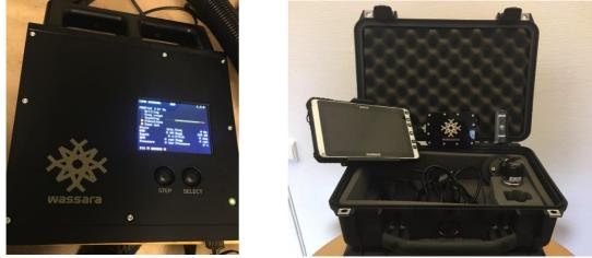
Figure 3. LKAB Wassara OWD® rig control unit and its field portable kit version.
